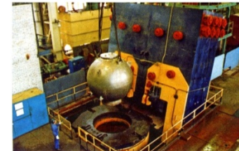
Chambers for hydraulic and hydrostatic tests
