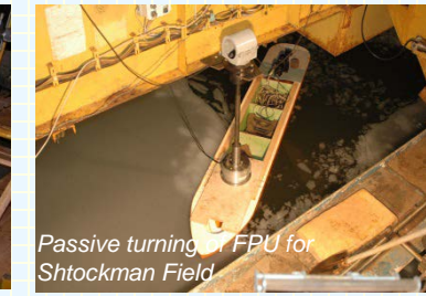
Model of SSFDR during seakeeping tests (Irregular seas)
