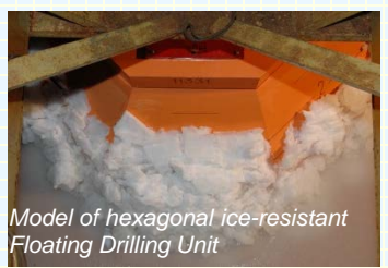
Interaction of SPAR model with level ice
