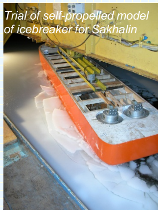
Towing and self-propelled tests of icebreaking vessel models in deep water and in shallow water and modeling interaction of propulsion/steering units with ice
