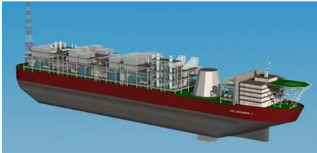
Offshore floating system for gas intake, preparation, and transfer from Shtokman field by pipelines to shore
