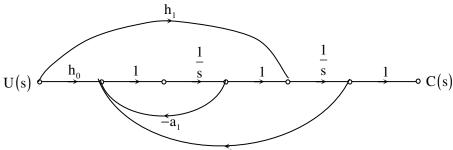
Assuming,  $h_1 = b_1$  and  $h_0 = b_0 - b_1$   $a_1$ , the input-output transfer function,  $G(s) = \frac{C(s)}{U(s)}$  of the
