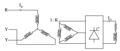
The converter is operated at a firing angle of 300. Assuming the load current (I0) to be virtually constant at 1 p.u. and transformer to be an ideal one, the input phase current waveform is
