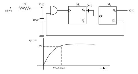
$\rightarrow$  given M<sub>1</sub> mono-stable multivibrator generates pulse width T<sub>1</sub>.
