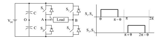
If the load current is sinusoidal and is zero at 0, x, 2x...., the node voltage  $V_{AO}$  has the waveform
