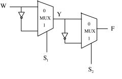
Output of first MUX =  $w \overline{s}_1 + \overline{w} s_1 = w \oplus s_1$ Let  $Y = w \oplus s_1$ Output of second MUX =  $Y \overline{s}_2 + \overline{Y} s_2$ =  $Y \oplus s_1$
