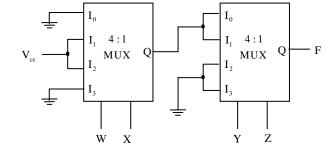
The output of the first MUX =  $\overline{W} \times V_{cc} + W\overline{X} \cdot V_{cc}$  $\overline{W}X + W\overline{X}$  (::  $V_{cc} = \log \operatorname{ic} 1$ ) =  $W \oplus X$
