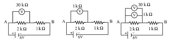
How will the three readings compare with one another if the potential drop were measured across the series combination of the  $2 k \Omega$  and the resistor i.e., across the points A and B?
