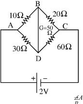
What is the current flowing in the  $\operatorname{arm}^{p}$ BD of this circuit? State the two laws used to find the current in different branches of this circuit.
