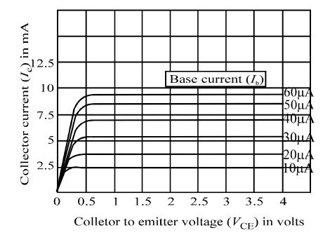
Use these graphs to estimate the value of the current amplification factor for the transistor for  $V_{CE} = 3V$ .
