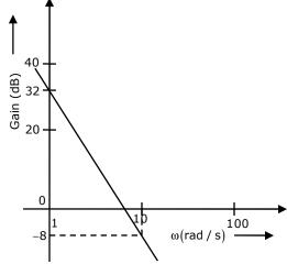
The gain  $(20 \log |G(s)|)$  is 32 dB and -8 dB at 1 rad/s and 10 rad/s respectively.
