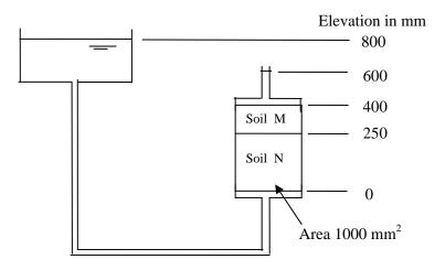
If the permeability of soil M is  $3 \times 10^{-4}$  mm s<sup>-1</sup>, the permeability of soil N, in mm s<sup>-1</sup>, will be
