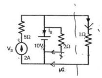
Q.50 The current in the  $1\Omega$  resistor in Amps is
