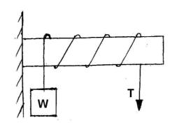
Determine the force required on the free end of the rope, to support a load of W = 20 kN. Take  $\mu$  as 0.30. (6)
