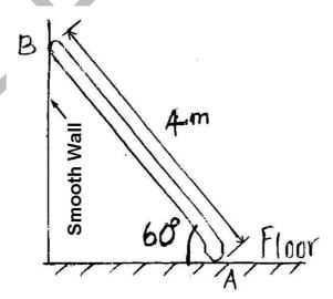
If a 750 N weight is applied at a distance of 3 m from the top of ladder, it is at the point of sliding. Determine the coefficient of friction between ladder and the floor. (10)
