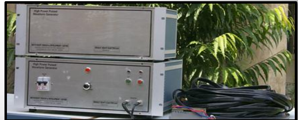
High Power (100kW peak) Pulsed Waveform Generator for turbo generator R-C Blocks testing at BHEL
