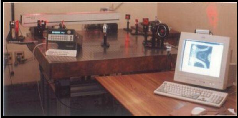
DSPI system for monitoring vibration and large deformations
