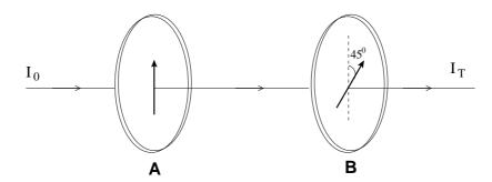
Assuming A and B to be perfect polarisers (i.e. no absorption losses), the intensity of the transmitted light will be  $I_T =$
