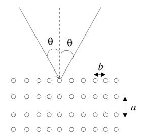
A condition for there to be a maximum in the diffracted X-ray intensity is
