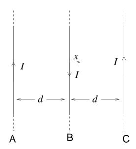
The wires carry equal currents I with directions as shown in the figure and have mass per unit length m. If the wires A and C are held fixed and the wire B is displaced by a small distance x from its position, then it (B) will execute simple harmonic motion with a time period
