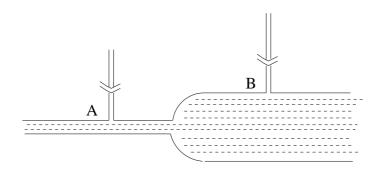
Two pressure gauges attached at the points A and B (see figure) show readings of  $P_A$ and  $P_B$  respectively. If the radius of the tube at the points A and B is 0.2 cm and 1.0 cm respectively, then the difference in pressure  $(P_B - P_A)$ , in units of dyne cm<sup>-2</sup>, is closest to
