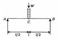
For the simply supported beam in the figure above, C is the centre of the span. C is also the point through which the resultant of the column load W passes. The column rests on the beam over a small length symmetrically on either side of C. What is the shearing force at C?
