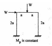
What is the ultimate load for the frame shown in the figure above ?
