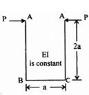
In the structure shown in the figure above, what is the distance through which the points A move towards each other?
