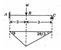
If a uniform beam shown in the figure above has the plastic moment capacity  $M_p$  for span AB and 0.9 Mp for span BC, what is the correct virtual work equation?
