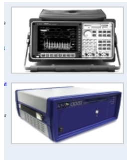
Dynamic Signal Analyser & Fibre Optic Based Strain Measurement System
