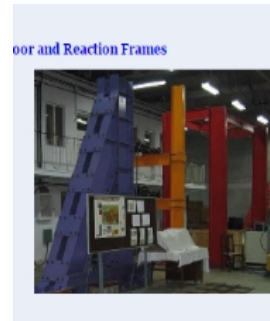
Structural Strong Floor Reaction Frames
