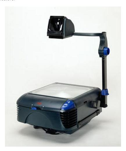
The OHP consists of a large box containing a very bright lamp and a fan to cool it, on top of which is a large lens. Above the box extends an arm with a mirror at its end. The lens focuses and redirects the light forward instead of up above.
