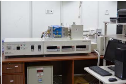
Seebeck Coefficient Measurement
