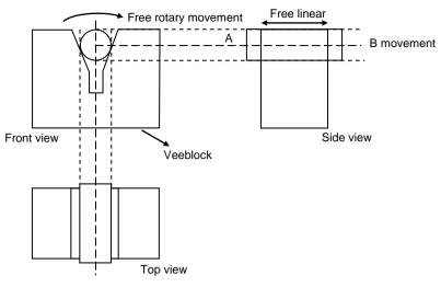
Figure 4.2 : Locating a Cylinder on a Vee Block
