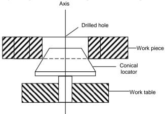
Figure 4.5 : Conical Locator
