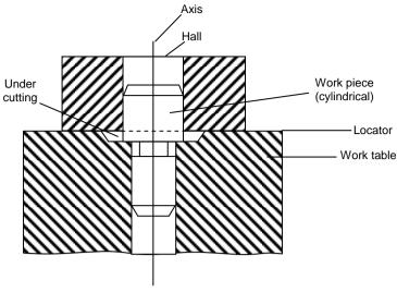
Figure 4.4 : Cylindrical Locator
