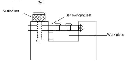
Figure 4.15 : Swinging Type Jig
