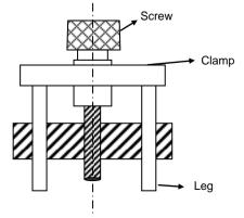
Figure 4.13 : Equalizing Clamp
