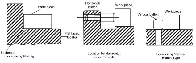
Figure 4.3 : Method of Locating using Flat Locators
