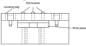
Figure 4.14 : Open Type Jig
