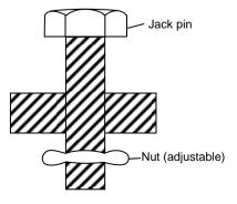
Figure 4.6 : Jack Pin Locator
