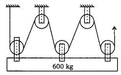
Which one among the following is the force required to move the mass of upwards? kg (a is acceleration due to gravity)
