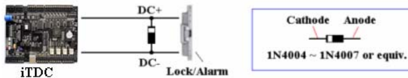
Figure : Reverse Diode connection
