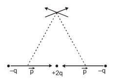
This system is behaving like two equal and opposste dipoles. So  $\vec{E}$  of both the dipoles will cancle each other.
