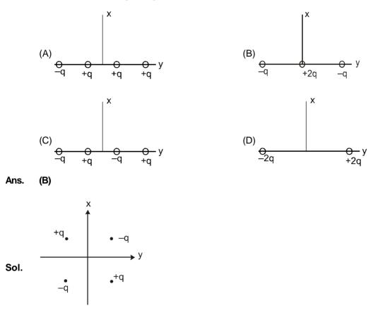
net  $\vec{E}$  due to all charges at a point on z- axis is zero. system B will produce zero  $\vec{E}$  at a far point on z axis
