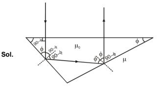
For given condition to be possible both  $\phi$  and 90° –  $\phi$  should be greater than critical angle  $\Rightarrow \qquad \mu_0 \sin \phi \ \ge \mu \sin 90^\circ$
