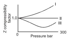
(A) I-ethene, II-oxygen, III- hydrogen
