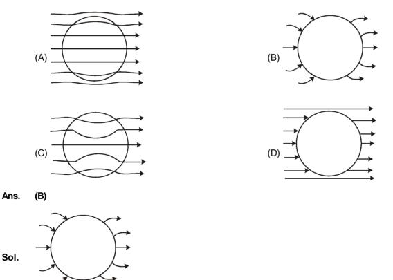
Electric field lines are always perpendicular to surface of conductor and absent inside the conductor.
