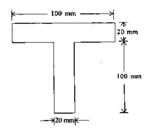
What is the distance between elastic neutral axis and plastic neutral axis for the cross-section as shown in figure above?
