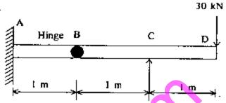
Which one of the following is the correct bending moment diagram for a propped cantilever beam shown in figure above?
