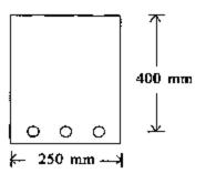
A simply supported RC beam having clear span 5 m and support width 300 mm has the cross-section as shown in figure. What is the effective span of the beam as per IS456?
