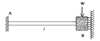
What is the bending moment at the end B for the guided beam as shown in the figure above considering the beam to be held rigidly at B against rotation and to support a load W?
