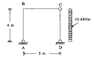
What is the value of vertical reaction at A for the frame shown in figure above?
