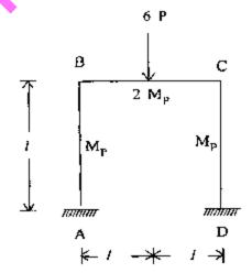
At the point of collapse, what is the value of horizontal thrust at point A in the loaded frame shown in figure?
