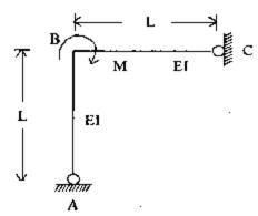
What is the rotation of the member at C for a frame as shown in figure above?
