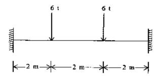
A beam of uniform section fixed at both ends and of span 6 m is acted upon by two concentrated loads of 6 t each as shown in figure above. What is the fixed end moment at each end?
