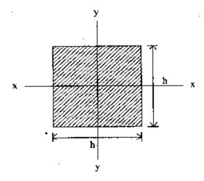
A square section as shown in the figure above is subjected to bending moment M. What is the maximum bending stress?
