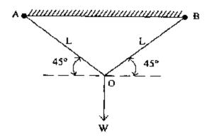
Two bars AO and BO are of uniform area 'A' and are hinged at O. What is the vertical deflection at O when elastic modulus is uniformly E?
