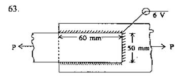
What is the safe load P that can be transmitted by the fillet-welded joint shown in figure above if the safe allowable shear stress in the fillet-weld is 108 MPa?
