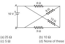
**25.** In the adjoining figure, if 10 calorie heat is produced per second in 5  $\Omega$  resistor due to the flow of current through it, then the heat produced in 6  $\Omega$  resistor is
