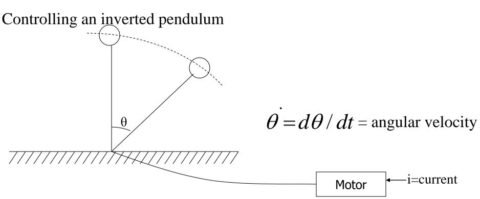
The goal: To keep the pendulum in vertical position ( $\theta$ =0) in dynamic equilibrium. Whenever the pendulum departs from vertical, a torque is produced by sending a current 'i'
