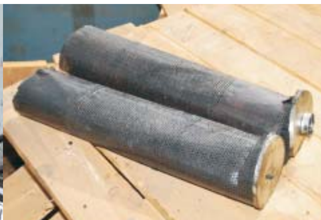
The pressed oil filters - ready to be fed in the furnaces
