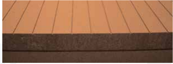
Photo 4. Vertical groove orientation running along the length of one side of the panel at 75mm spacings.
