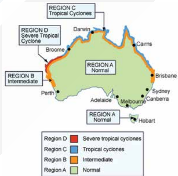
Figure 1. Wind Region designation around Australia. Refer to the BCA table 1.1.1 Design Wind Speed-Equivalent Values for more information.
