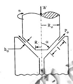
A hydrostatic conical thrust bearing is shown in the figure. Show that the load carrying capacity of the bearing is given by
