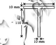
For the depth of plastic neutral axis from the top of the T-section to be 9.583 mm, the flange width b must be
