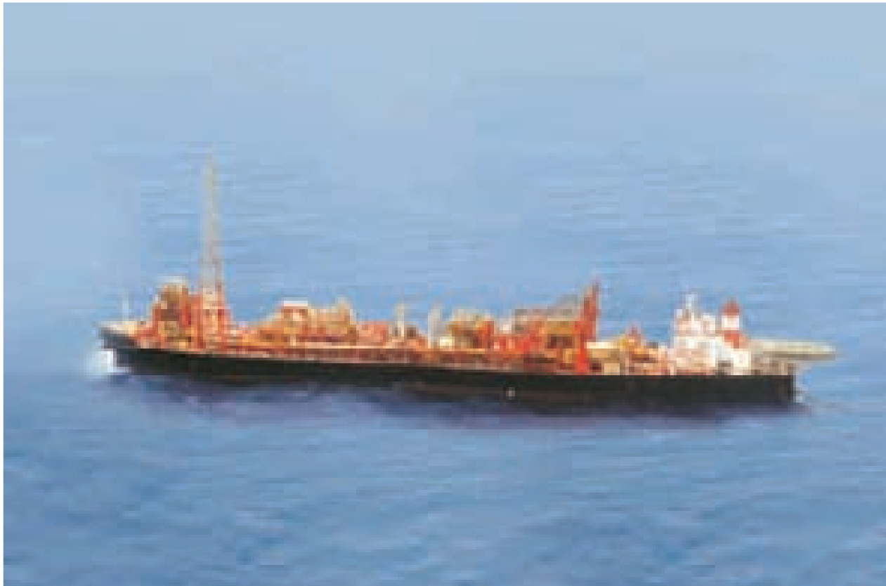
An FPSO (Floating Production Storage and Offloading vessel) unit; ONGC has taken a slew of initiatives to quickly put its fields on production using the latest state-of-the-art technology. The induction of FPSO units to its fleet has greatly advanced the production schedule in the eastern offshore.
