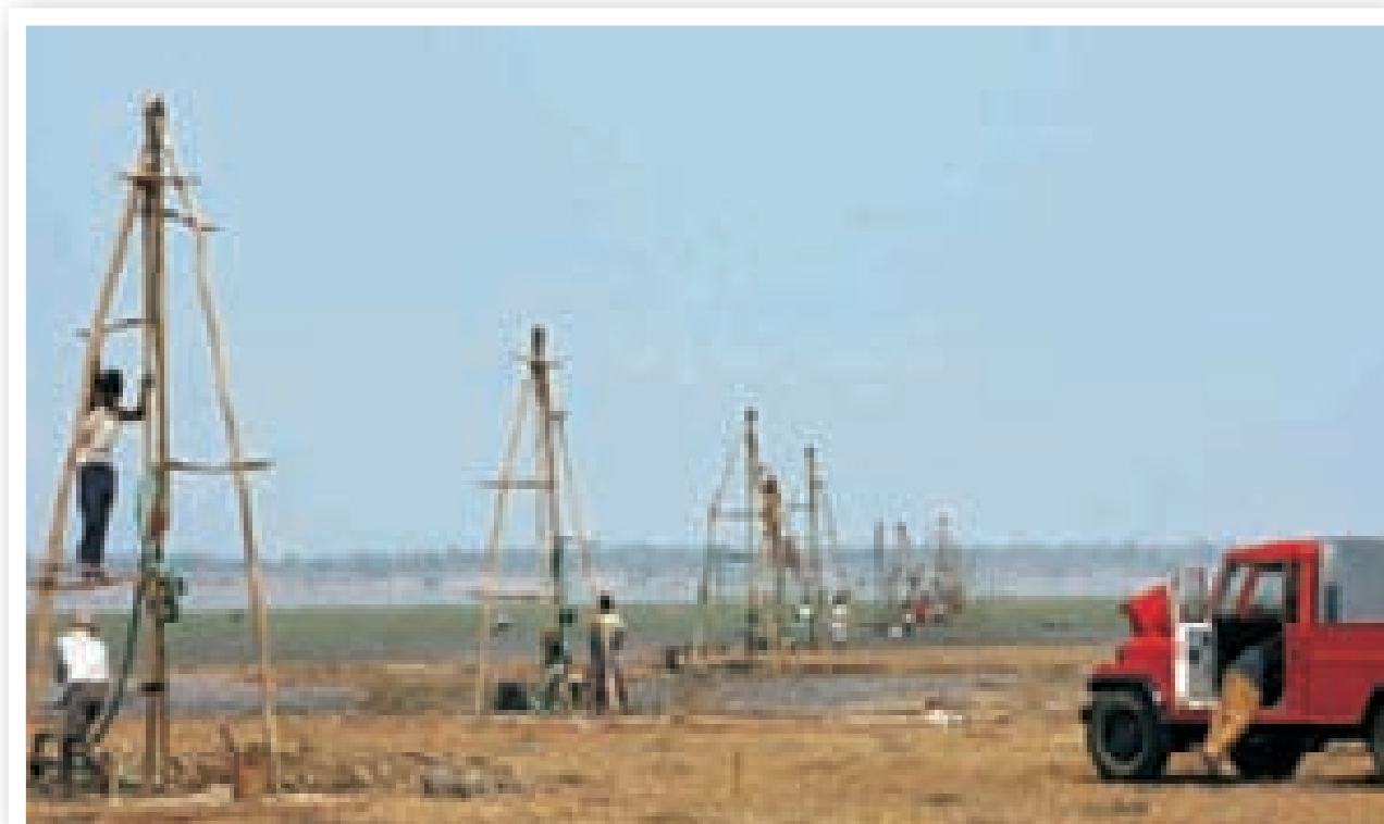
Preparation of shot-hole drilling for seismic survey; ONGC made 22 new discoveries in FY'15 - 10 new prospects and 12 new pools
