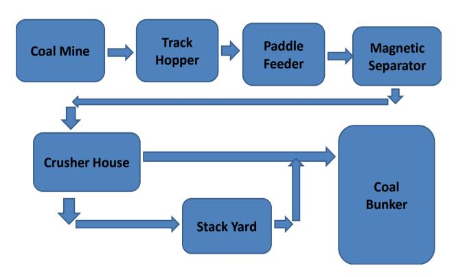
At power plant, coal is unloaded in track hoppers of length 200-250m normally. The unloading mechanism used in NTPC is Bottom Open Box type Rake (BOBR).
