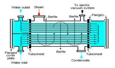
Condenser is basically a heat exchanger which condenses a steam and converted into water. After expansion of steam in LP turbine it enters in the condenser. In condenser there are many water tubes are provided to condensate the steam.
