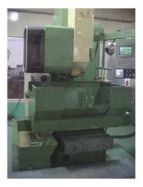
Fig. 1.3 A CNC Machine with an Automated Tool Changer and the Operator Console with Display for Programming and Control of the Machine
