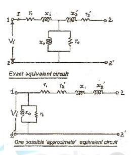
$I_0$  'Shall be slightly greater than  $I_0$  and therefore, slightly greater core loss Current flowing through  $r_1$  is now somewhat less than  $I_1$  and therefore reduced copper loss in it
