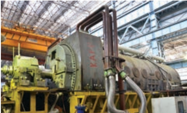
First 700 MW Nuclear Turbo Generator set under testing on test bed
