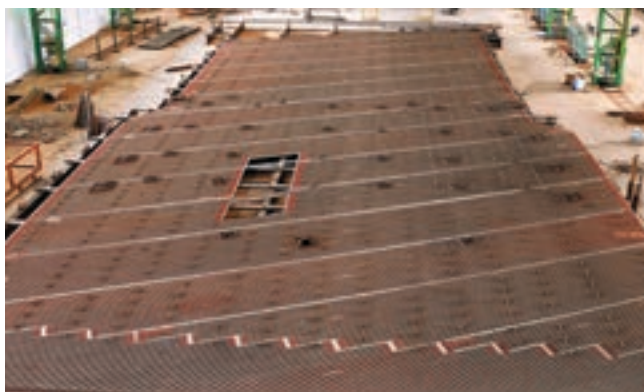
Spiral Furnace wall panel for 660 MW Supercritical boilers manufactured at HPBP, Trichy
