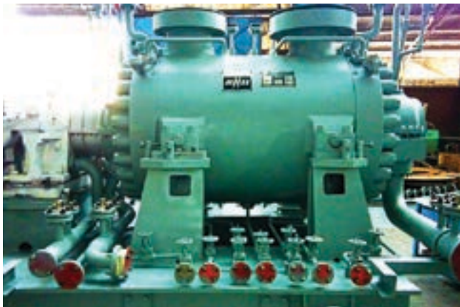
Multi-stage centrifugal compressor manufactured & supplied by BHEL
