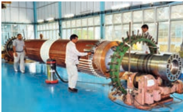
800 MW Turbo Generator rotor under assembly at HEEP, Haridwar
