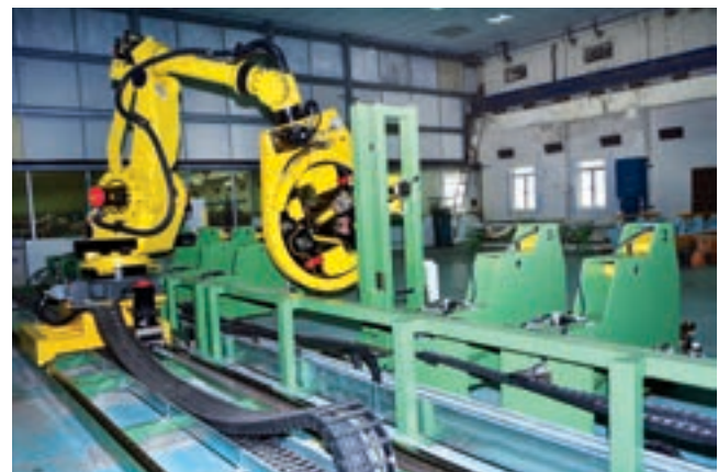
CNC 6 Axis Taping machine installed at HPEP, Hyderabad for enhancing Turbo Generator manufacturing capability
