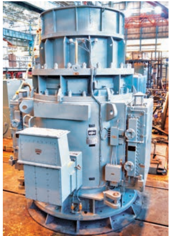
6 MW, 6.6 kV Primary Coolant Pump Motor
