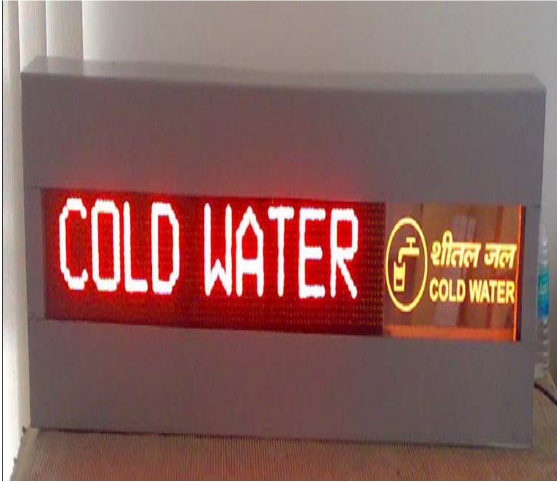
FIGURE 1: Images of Variable cum Fixed message signage system
