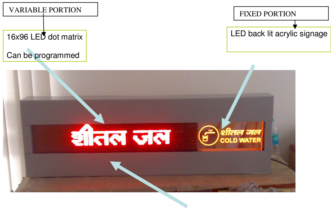
FIGURE 2: ACP body for extended durability finish for Variable cum Fixed message signage system
