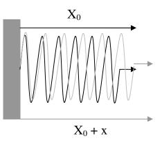
Now, consider molecules where real chemical bonds exist. For simplicity and convenience one can assume that the vibrational motion of the chemical bonds to be harmonic and thus want to find the energy associated with the vibrational motion of the molecular bonds. Consider, for example, a carbon-carbon bond. The bond stretched and compressed between an equilibrium distance of  $R_0$  to  $R_0 \pm r$ , where r is the extent of stretching (compression).
