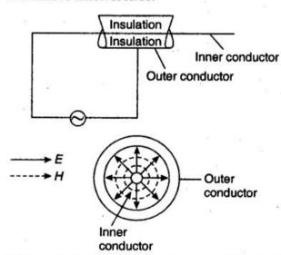
Different kinds of dielectric materials, such as teflon and polythene are covered over copper wire, it acts as a spacer.
