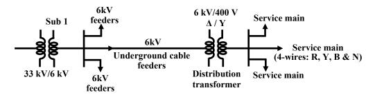
Figure 2.11: Typical Power distribution scheme.
