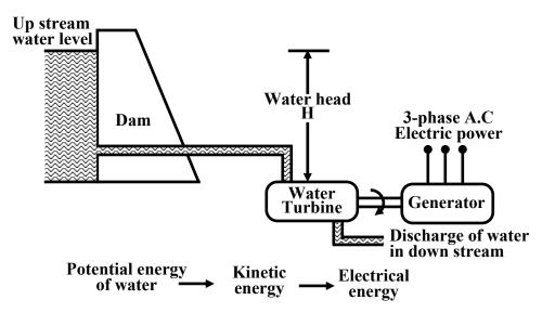
Figure 2.3: Basic components of a hydel generating unit.
