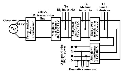
Figure 2.6: Typical voltage levels in a power system.
