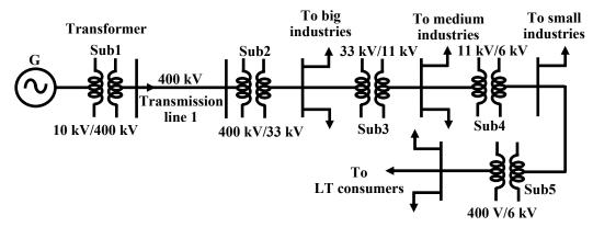
Figure 2.9: Single line representation of power system.
