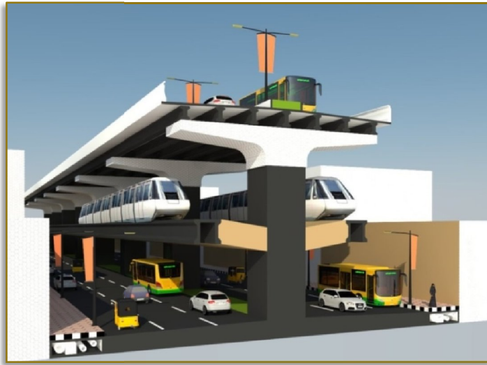
Model cross section for the skyway with Metro Rail integration
