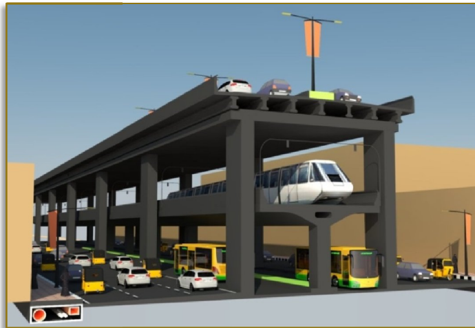
Model cross section for the skyway above Metro Rail
