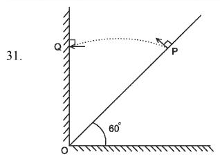
From point P, a particle is projected with a velocity of 40 m/s perpendicular to the inclined plane and also strikes perpendicularly at point Q. Find the time taken by the particle in moving from P to Q.
