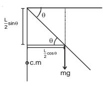
Loss in Potential Energy = gain in Kinetic Energy, mg  $\frac{L}{2}\sin\theta = \frac{1}{2}I\omega^2$ ,  $\omega \propto \sqrt{\sin\theta}$ ,  $v \propto \sqrt{\sin\theta}$
