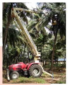
The time required for locating unit and operating stabilizers was 1 min. The time required for positioning against a tree of 10 m height was 2 min. Suitable safety devices were incorporated to ensure stability of the hoist. The positioning of the operator platform can be done by the operator himself using electro hydraulic controls.
