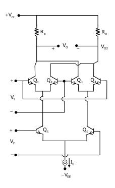
For the circuit shown in the above figure determine by relevant analysis, under what conditions the output voltage is proportional to the multiplication of the two inputs  $V_1$  and  $V_2$ . Derive an expression for  $V_0$  in terms of  $I_B$ ,  $V_1$  and  $V_2$ .
