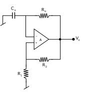
Assuming the gain A of the op-amp to be represented by  $A = \frac{\omega_t}{s}$  where  $\omega_t$  is the gain bandwidth-product of the op-amp, analyze the given circuit and determine under what condition, the circuit can generate sinusoidal signal at the output? What is the frequency of the output waveform if  $R_1 = 1K\Omega$ ,  $R_2 = 9K\Omega$ ,  $C_o = 0.1\mu F$  and  $R_o = 10K\Omega$ ?
