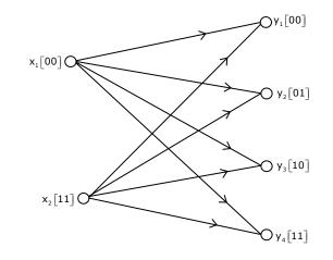
Calculate the rate of joint information transmission for the above channel. Assume  $p(x_1) = p(x_2) = \frac{1}{2}$  where  $[X] = \{x_1, x_2\}$  is the set of input symbols. Assume  $q \rightarrow$  Probability of correct reception. P= Probability of incorrect reception and  $[Y] = \{y_1, y_2, y_3, y_4\}$  be the set of received symbols.
