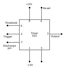
In the IC Timer 555 shown in the above figure determine the reference levels for the two comparators inside the chip. Justify your answer by drawing a block diagram of the internal circuit of IC Timer 555.
