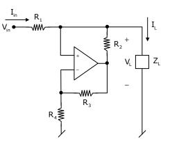
Explain the operation of the circuit shown in the above figure and determine under what condition the output current  $(I_L)$  can be made independent of load voltage ?
