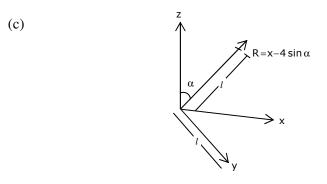
A V-shaped antenna is shown in the above figure. The current distribution on the antenna is given by  $I = I_0 \cos(K_0 u)$  and the length of the antenna is 1.
