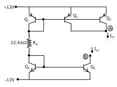
Assuming matched transistors with large  $\beta$  (i.e., negligible base currents), determine the currents  $I_{o1}$  and  $I_{o2}$  in the circuit given in the above figure. Assume that nodes (B) and (A) are connected at appropriate voltages which ensure the transistors  $Q_5$ ,  $Q_2$  and  $Q_3$  are in active region.
