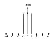
(D) Periodic discrete time signal consisting of 3 non-zero samples
