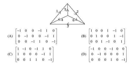
107. For the oriented graph as given above, taking 4, 5, 6 as tree branches the tie set matrix is
