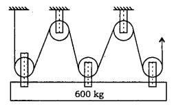
Which one among the following is the force required to move the mass of 600 kg upwards? (g is the acceleration due to gravity)
