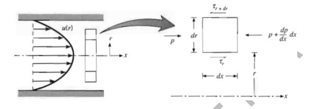
> For the annular differential element, force balance will be reduced to:
