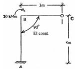
The figure given above shows a rigid frame fixed at A and hinged at C. If a pure moment of 20 kNm is applied at B in the plane of the figure, then what is the moment at the fixed end A?
