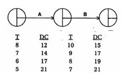
Two activities A and B are to be done in the given sequence. The variation of direct cost (DC) with possible activity duration (T) (in days) is indicated for each activity above. What is the increase in total direct cost between a combined duration of 16 days and 13 days?
