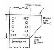
Which one of the following is the most critical rivet in the joint shown in the figure given above?
