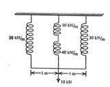
What is the equivalent spring stiffness for the system of springs shown in the figure given above?
