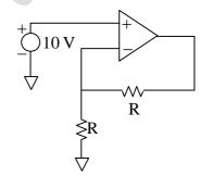
The non-inverting input is connected to a DC voltage of +10V. The voltage at the inverting input will be
