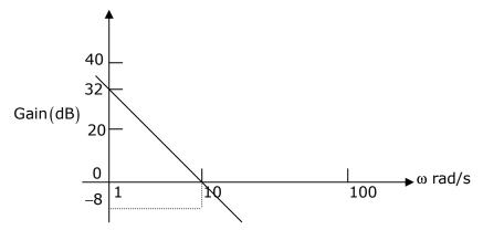
The gain (20 log |G(s)|) is 32dB and -8dB at 1 rad/s and 10 rad/s respectively. The phase is negative for all  $\omega$ . Then G(s) is
