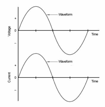
Fig. 3: In Phase Voltage and Current Signals
