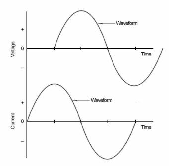
Fig. 6: Negative Reactive Power - Voltage Lags Current
