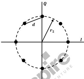
52. For the constraint that the minimum distance between pairs of signal points be d for both constellations, the radii  $r_1$  and  $r_2$  of the circles are
