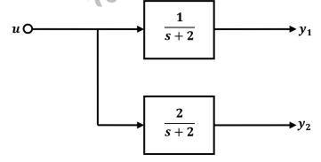
A state space model of the above system in terms of the state vector x and the output vector  $y = [y_1 \quad y_2]^T$  is
