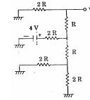
What is the output voltage ' $V_0$ ' of the R-2R decoder ladder network?
