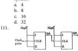
The above circuit illustrates a typical application of the JK flip-flops. What does this represent?
