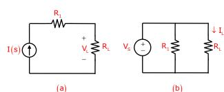
$\rightarrow$  From figure (a), observe that if we keep or remove R<sub>1</sub> the load voltage and current are same so  $R_1$  is redundant here
