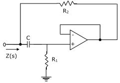
12. Find the value of R' in the circuit of Fig.12 for generating sinusoidal oscillations. Find the frequency of oscillations.
